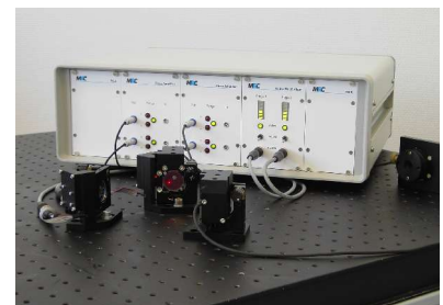
Setup of Dynamic beam alignment (2-mirror alignment)
