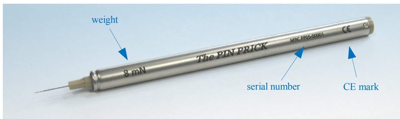
Figure 5: Marking of a PinPrick stimulator
